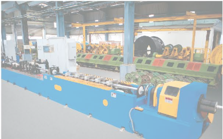
Aluminium Corrugation Sheathing Line
