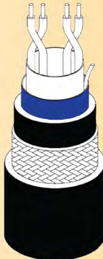
OVERALL SCREENED INSTRUMENT CABLE
