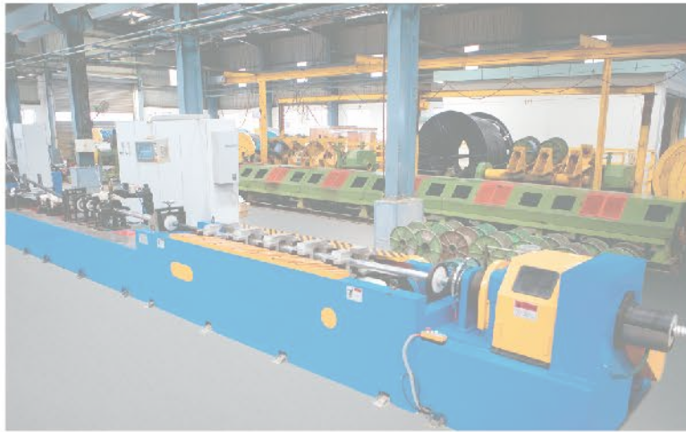
Aluminium Corrugation Sheathing Line
