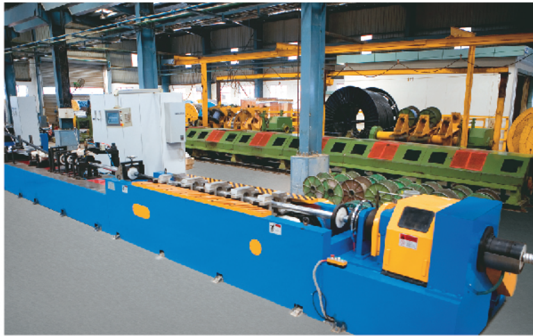
Aluminium Corrugation Sheathing Line
