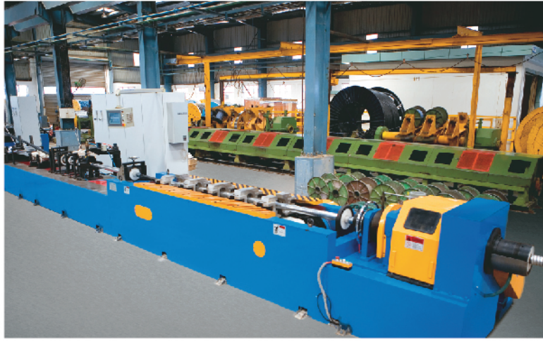
Aluminium Corrugation Sheathing Line
