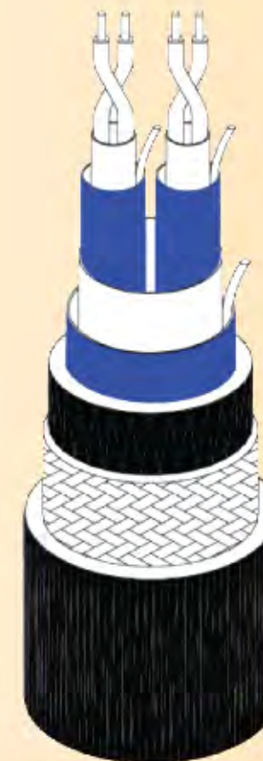
INDIVIDUAL & OVERALL SCREENED INSTRUMENT CABLE
