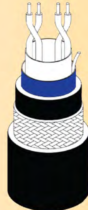
OVERALL SCREENED INSTRUMENT CABLE
